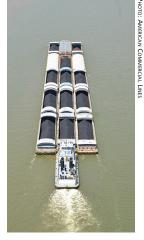
A barge tow primarily consisting of coal in open hopper barges, each with a capacity of approximately 2,000 tons.
