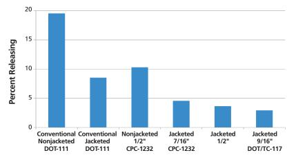
FIGURE 2 Percentage of tank cars of various designs expected to release 100 or more gallons (CPR<sub>100</sub>) from physical impacts in FRAreportable accidents (4).
