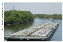
Typical liquid barge tow for products such as ethanol and petroleum. Each of the six barges in this photo carries 30,000 barrels, or 4,200 tons, of product. world markets. Ethanol plants tend to draw corn from within a 50-mile radius, establishing local markets. Distillers dry grains, a byproduct of the ethanol distillation process, regularly move by barge to the export market or to domestic markets for animal feed.
