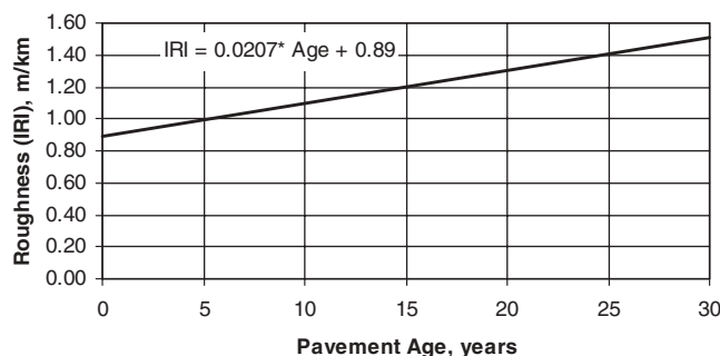
Figure 13. Assumed roughness do-nothing curve for Case Study 1—Arizona.
