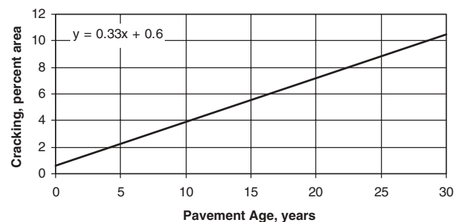
Figure 15. Assumed cracking do-nothing curve for Case Study 1—Arizona.
