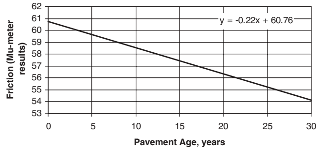
Figure 14. Assumed friction do-nothing curve for Case Study 1—Arizona.
