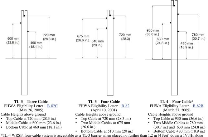
\*TL-4 WRSF, four-cable system is acceptable as a TL-3 barrier when placed no further than 1.2 m (4 feet) down a 1V:4H slope (for adjacent traffic impacts) and no closer than 3 m (10 feet) from the ditch bottom for opposite-side impacts (FHWA B-82-B).
