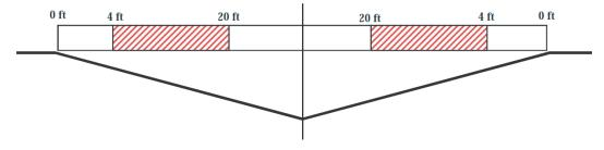
FIGURE 3 Override criteria for V-shaped medians steeper than a 6H:1V slope (Figure 6.2 from *NCHRP Report 711*) (Marzougui et al. 2012).
