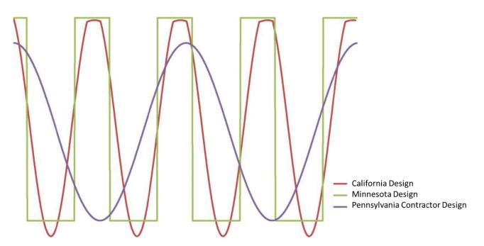
FIGURE 10 Comparison of rumble strip cross sections (Minnesota, California, and Pennsylvania) (Terhaar 2015).
