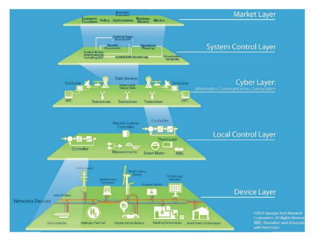
FIGURE 3-3 Cyber-physical infrastructure of the smart grid.
