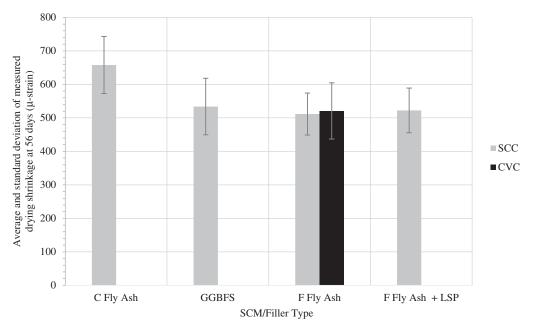
*Figure 2-30.* Average and standard deviation of measured 56-day drying shrinkage for CVC and SCC mixtures.
