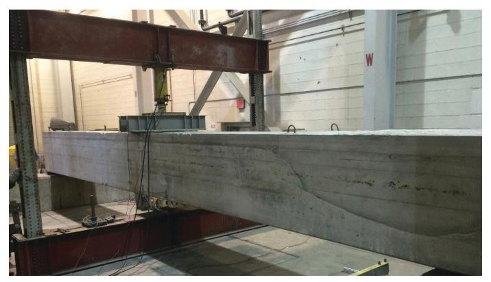
Figure 1-20. Setup of the flexure test of box girder specimen.
