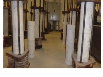
Figure 1-13. Creep test setup.
