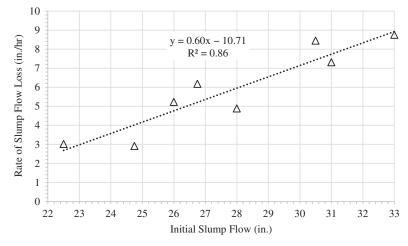
Figure 2-9. Initial slump flow versus rate of slump flow loss.
