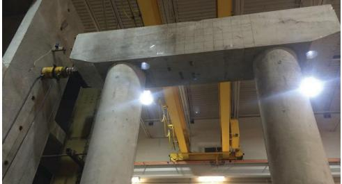
Figure 1-19. Column test setup.
