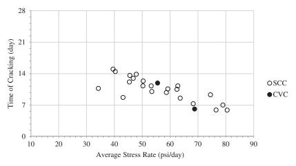
*Figure 2-31. Restrained shrinkage test data for SCC and CVC mixtures.*
