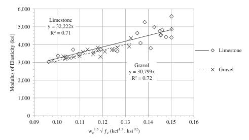
*Figure 2-16.* Comparing MOE of SCC mixtures containing gravel and *limestone aggregates.*
