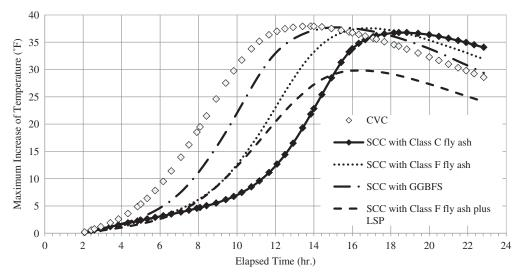
*Figure 2-12. Semi-adiabatic calorimetry test results for mixtures containing* ½ *in. nominal maximum size limestone aggregates.*
