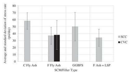
Figure 2-32. Average and standard deviation of stress rate for CVC and SCC mixtures with different types of SCM/filler.
