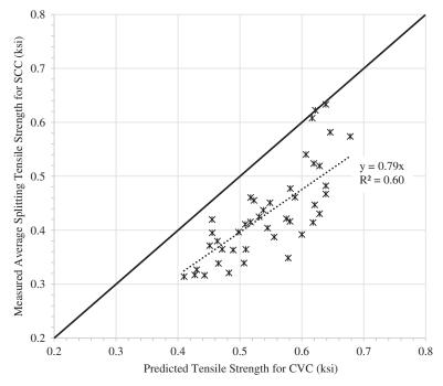
Figure 2-18. AASHTO predicted tensile strength for CVC versus measured tensile strength for SCC.
