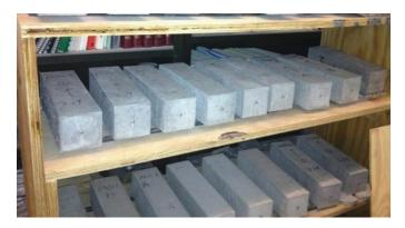
Figure 1-11. Drying shrinkage specimens.
