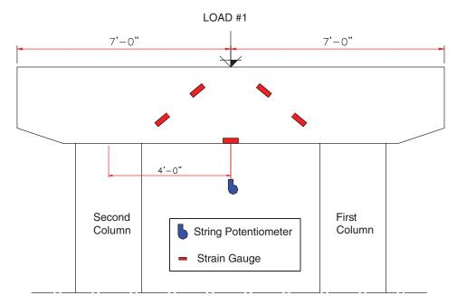
Figure 1-18. Pier cap test setup.
