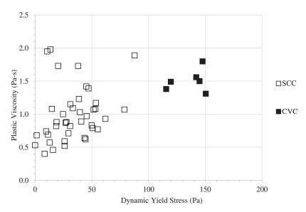
Figure 2-1. Rheological properties of mortar mixtures.
