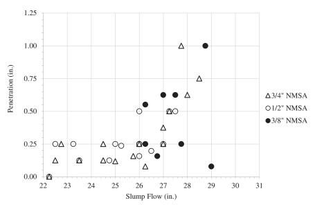
Figure 2-6. Penetration versus slump flow.
