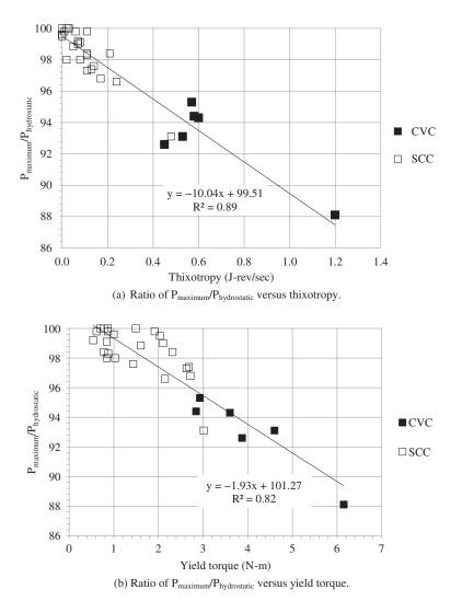
Figure 2-10. Ratio of P<sub>maximum</sub>/P<sub>hydrostatic</sub> versus thixotropy and yield torque.
