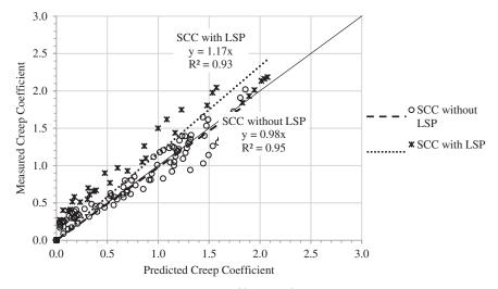
*Figure 2-34. Predicted creep coefficient for CVC versus measured creep coefficient for SCC mixtures.*
