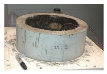
Figure 1-12. Restrained shrinkage specimen.
