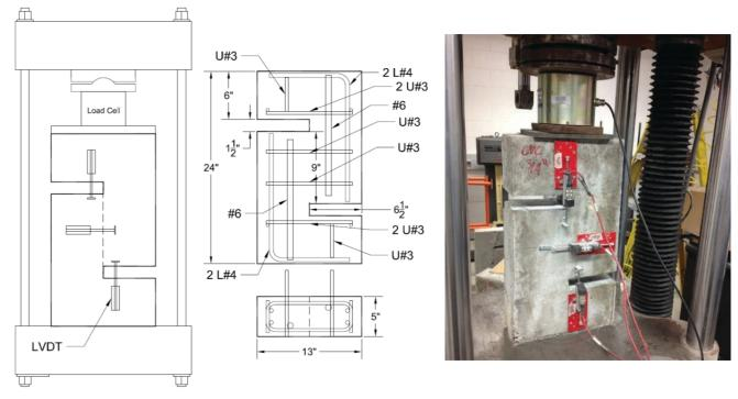
Figure 1-9. Push-off test setup.
