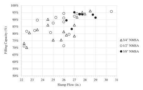
Figure 2-5. Caisson filling capacity of SCC versus slump flow.
