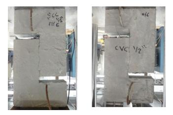
*Figure 2-23. Interface shear cracking of SCC and CVC push-off specimens.*
