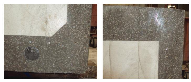
Figure 2-44. Saw cut in the bridge box girder specimen showing top and bottom corners.
