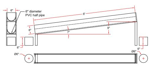
Figure 1-5. Modified flow trough used for evaluating dynamic stability.
