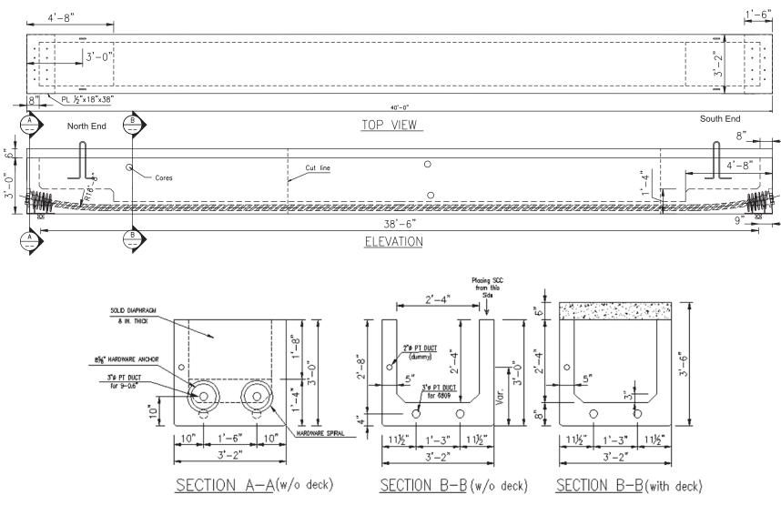
Figure 1-16. Views of the bridge post-tensioned box girder specimen.
