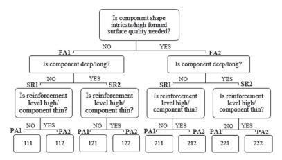
Figure 1-3. Process for determining workability targets.
