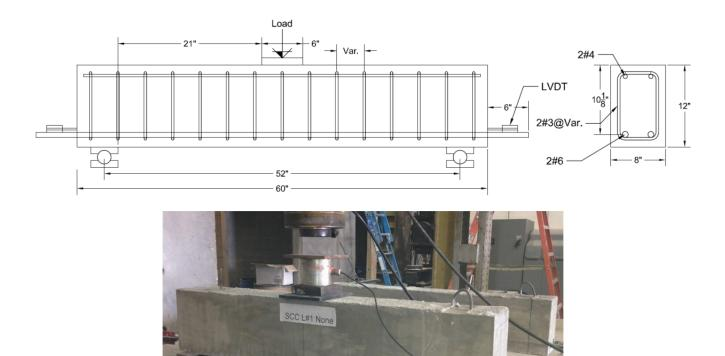
Figure 1-10. Beam shear test setup.
