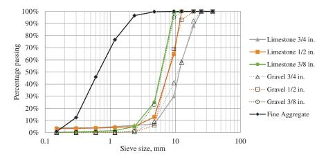
Figure 1-2. Particle size distribution of fine and coarse aggregates.
