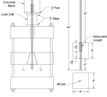
Figure 1-7. Pull-out test setup.
