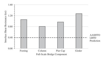
*Figure 2-25. Interface shear resistance of unreinforced SCC push-off specimens.*
