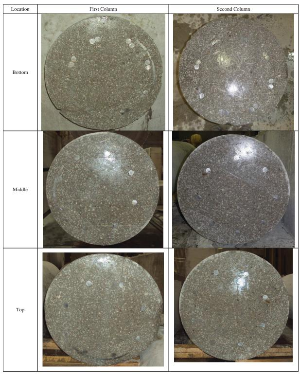
*Figure 2-41. Saw cuts at the bottom, middle, and top of the two pier columns.*
