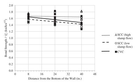
*Figure 2-21. Top-bar effect on bond strength of horizontal bars in CVC and SCC mixtures.*
