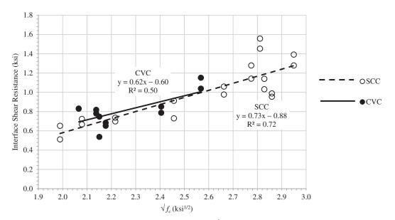
Figure 2-22. Interface shear resistance versus  $\sqrt{f_c}$  of SCC and CVC mixtures.
