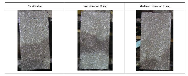
Figure 2-45. Saw cuts of three cylinders with different levels of vibration.
