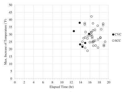
Figure 2-11. Maximum increase of temperature in semi-adiabatic condition.
