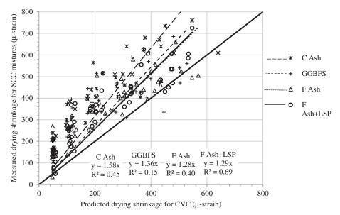
*Figure 2-29. AASHTO LRFD predicted drying shrinkage for CVC versus measured drying shrinkage for SCC mixtures.*
