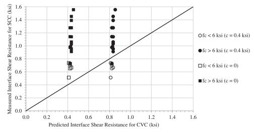
Figure 2-24. Measured interface shear resistance for SCC versus that predicted by AASHTO LRFD for CVC.
