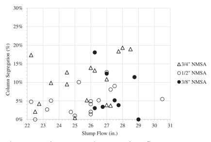
Figure 2-7. Column segregation versus slump flow.
