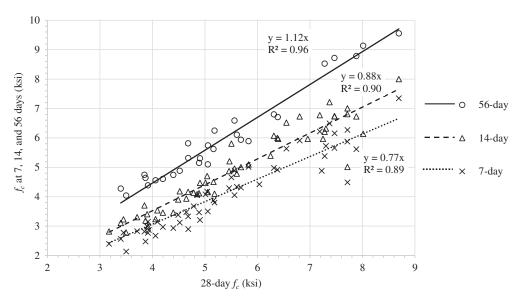
Figure 2-15. Relationships between average compressive strength at 7, 14, and 56 days and average compressive strength at 28 days for SCC mixtures.
