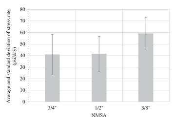
Figure 2-33. Average and standard deviation of stress rate for SCC mixtures with different NMSA.
