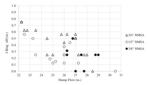
Figure 2-4. J-ring difference in average height ( $\Delta H$ ) versus slump flow.
