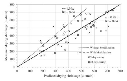
Figure 2-39. Measured versus predicted drying shrinkage for SCC mixtures.
