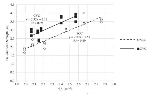
*Figure 2-20.* Pull-out bond strength versus  $\sqrt{f_c}$  of SCC and CVC mixtures.
