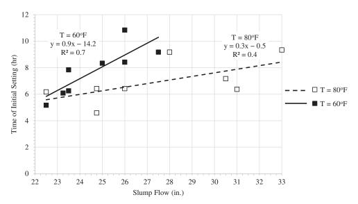
Figure 2-14. Time of initial setting versus slump flow for SCC mixtures.
