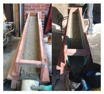
Figure 1-4. Original (left) and modified (right) flow troughs used for evaluating dynamic stability.
