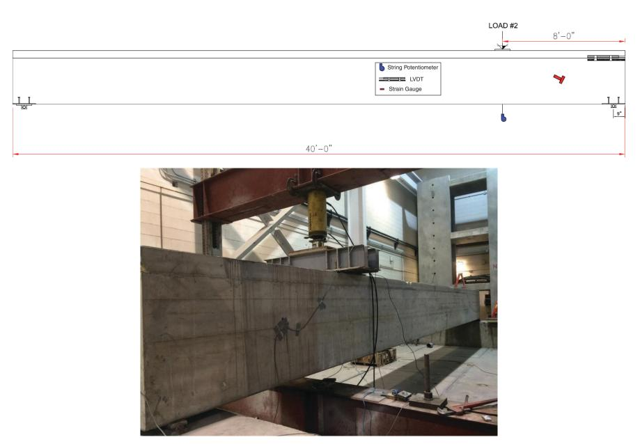
Figure 1-21. Setup of the shear test of box girder specimen.
