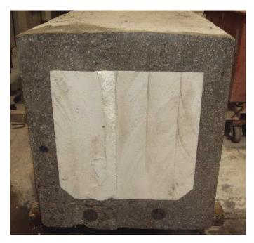
Figure 2-43. Saw cut in the bridge box girder specimen.
