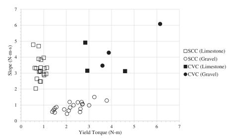
Figure 2-2. Rheological properties of concrete mixtures.
