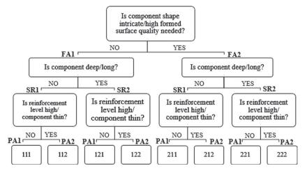
Figure B-2. Decision tree used to determine workability targets.
