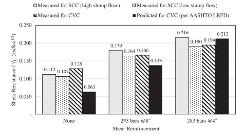
*Figure 2-26. Shear resistance of SCC and CVC mixtures with different reinforcement.*
