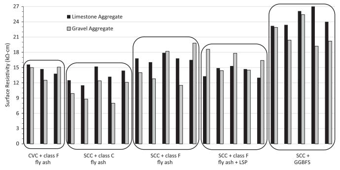
Figure 2-36. Surface resistivity of SCC and CVC mixtures.
