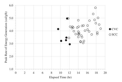
*Figure 2-13. Peak rate of energy generation in isothermal condition.*
