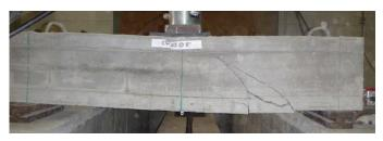
(a) Shear cracking in a CVC beam.
