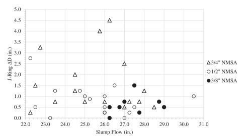
Figure 2-3. J-ring reduction in slump flow diameter ( $\Delta D$ ) of SCC versus slump flow.
