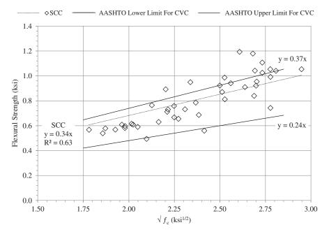
Figure 2-19. Average measured flexural strength of SCC mixtures versus square root of average 28-day compressive strength.
