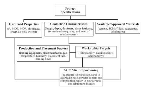
*Figure B-1. General steps of proportioning SCC mix for cast-in-place bridge components.*
