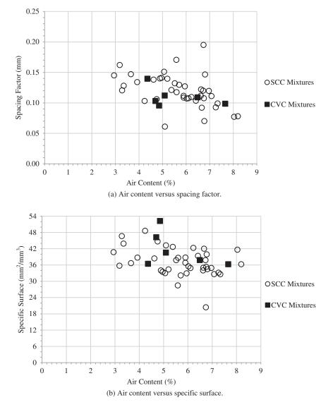
Figure 2-35. Air void system parameters for hardened SCC and CVC.
