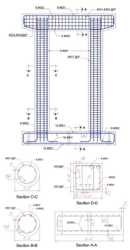
Figure 1-15. Reinforcement details and cross sections of the bridge pier specimen.
