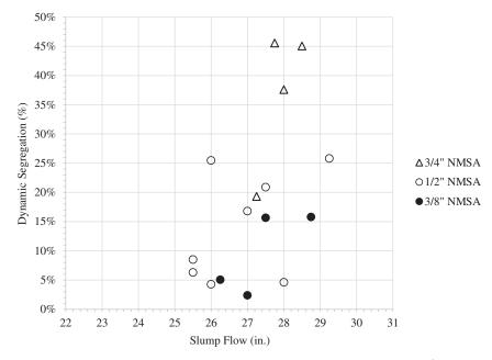
Figure 2-8. Flow trough dynamic segregation versus slump flow.
