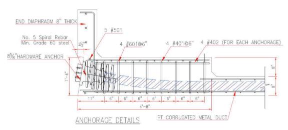
Figure 1-17. Reinforcement details of the box girder specimen.
