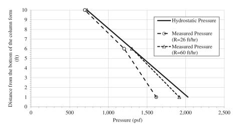
Figure 2-38. Measured SCC formwork peak pressure for different placement rates.
