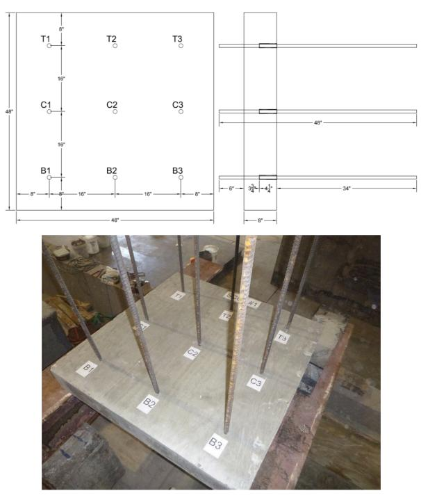
Figure 1-8. Details of wall-out wall specimens.
