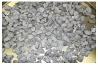
Manually separated No. 6 Stone with limited evidence of RAP binder transfer
