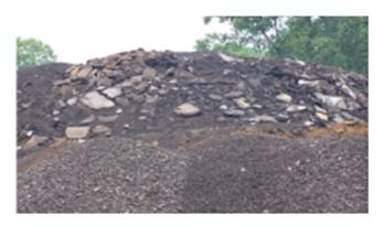
FIGURE 18 Example of RAP from variations in RAP materials from various sources [demolition (*top, center*) and millings from different projects (*bottom*)] (*Source*: West 2010).
