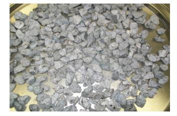
FIGURE 36 Appearance of No. 6 limestone after dry mixing with RAP in laboratory pugmill (*Source*: Hines 2015).
