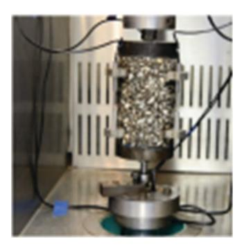
FIGURE 13 Repeated direct tension test (*Source*: NCHRP 9-57 Workshop 2015).
