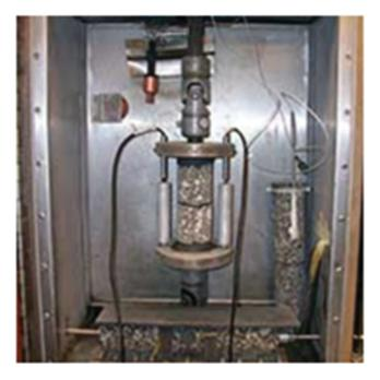
FIGURE 16 Thermal stress restrained specimen test set up (*Source*: Western Regional Superpave Center [Online]. http://www.unr.edu/wrsc/research/facilities/asphalt).
