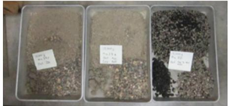
FIGURE 41 RAP transfer to virgin aggregate in laboratory pugmill (*Source*: Johnson et al. 2013).
