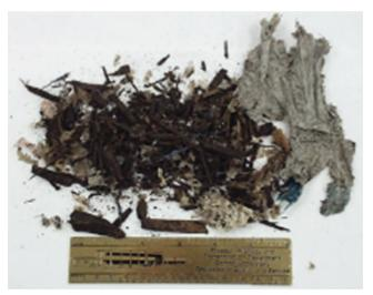
When deleterious materials (contaminates) are not removed from the RAS supply, they are ground up along with the shingles
