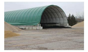
FIGURE 17 Covering stockpiles helps control the moisture content (*Source*: Jackson 2012).
