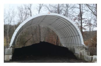
FIGURE 35 Cover stockpiles to minimize moisture content (*Source*: Jackson 2012).
