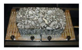
FIGURE 12 Overlay tester for evaluating reflective cracking resistance (*Source*: Klutzz and Mogawer 2012).
